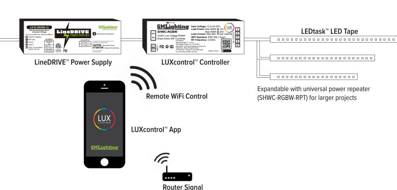
**Note:** For use with LD-E (non-dimmable) or LD-ED (dimmable) power supply only. Not compatible with LD-MD (magnetic) power supply.
